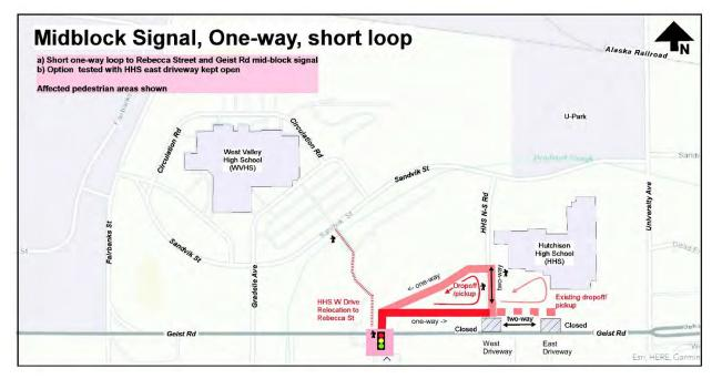
Figure 27. Signal, Midblock, one-way short frontage loop option (HHS)
