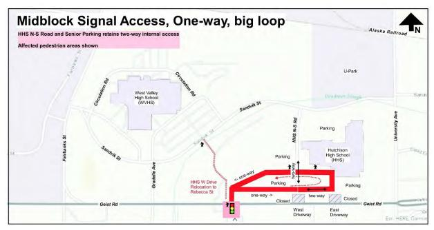
Figure 33. Signal, Midblock, one-way long frontage loop option (HHS)
