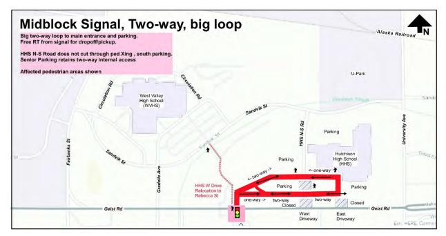
Figure 35. Signal, Midblock, two-way short frontage loop option (HHS)
